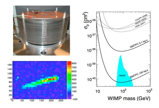
**Figure 1:** Top left: image of the 10-liter DMTPC prototype. Bottom left: image of a nuclear recoil from a low-energy neutron in  $CF_4$  at 75 torr. Right: expected sensitivity (90% C.L.) to spin-dependent WIMP scattering on protons for a DMTPC detector (solid lines) compared with published limits from other experiments (dashed lines). The shaded area shows the MSSM favored region.
