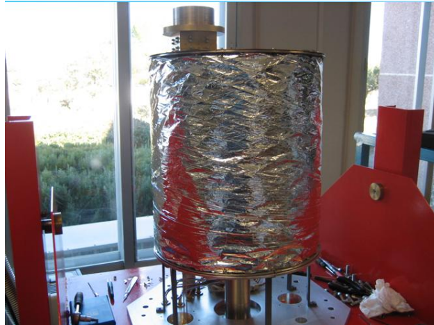
Figure 7: Example of MLI in an intermediate stage of a cryostat
