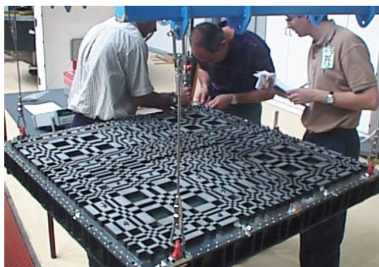
Figure 1: The IBIS mask containing four repeats of the basic pattern
