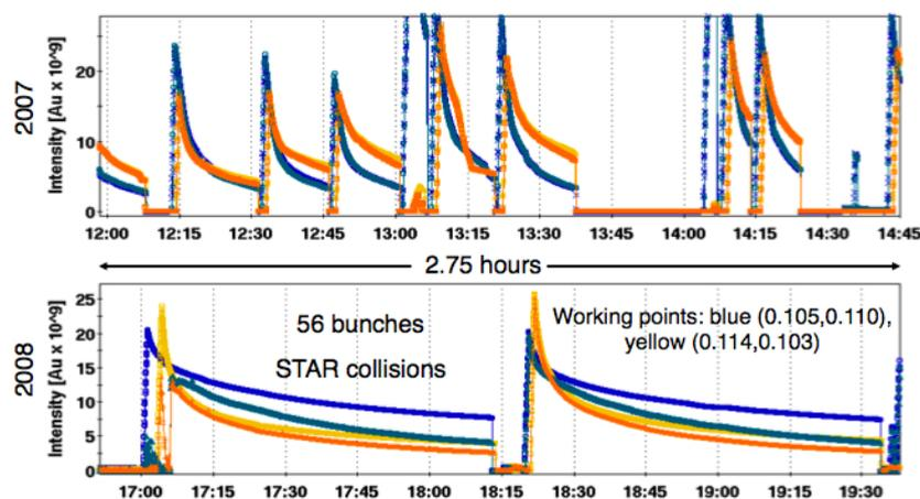
**Figure 1:** Comparison of 2007 (top) and 2008 (bottom) beam lifetimes at  $\sqrt{s}=9.18$  GeV/n. Traces show circulating total and bunched beam intensities in correspondingly-colored RHIC rings. Sextupole reversal and elimination of strong octopoles clearly improved beam lifetime.
