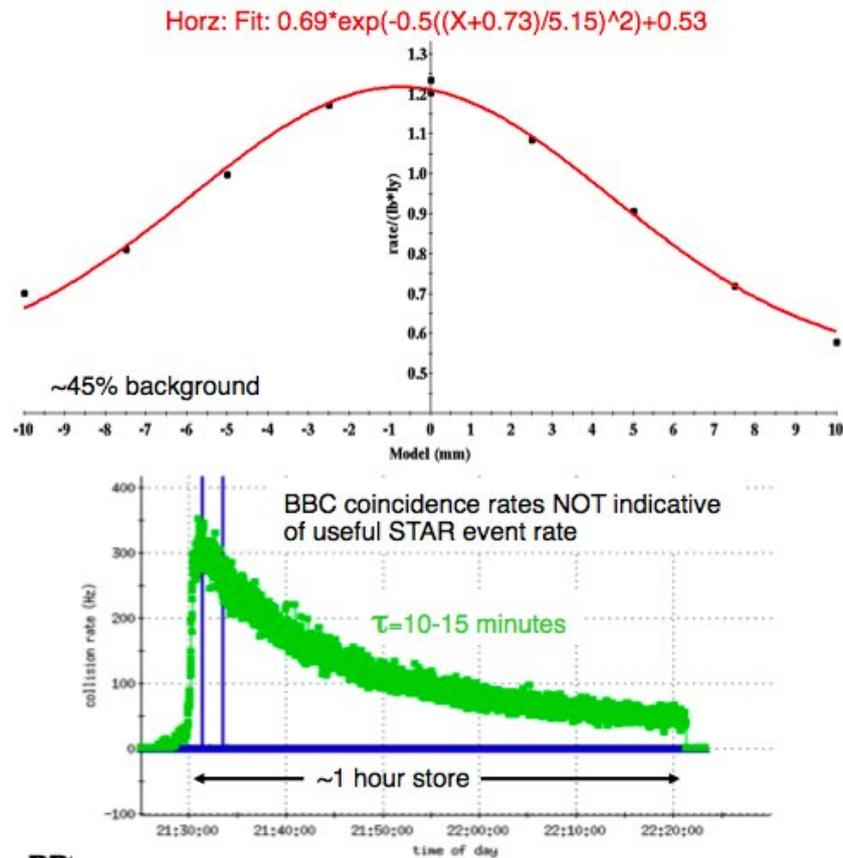
**Figure 2:** A horizontal vernier scan at the STAR detector during  $\sqrt{s}=9.18$  GeV/n operations, and beam-beam counter (BBC) luminosity evolution during a typical store. Collision rate scaling was incorrect in this picture; actual event rates were on the order of 1 Hz.
