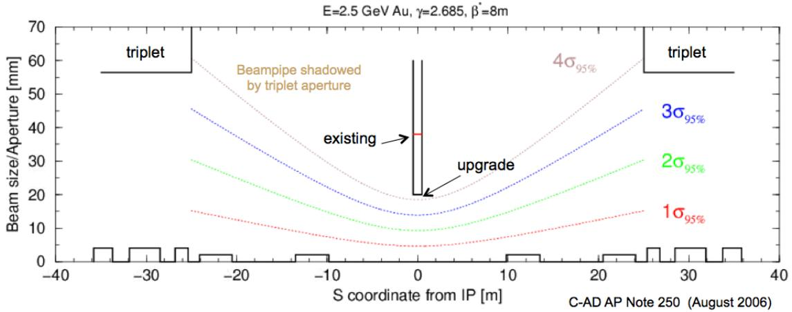
**Figure 4:** Beam size and aperture limitations in a RHIC IR, showing existing and upgrade beampipe apertures for gold beam with normalized emittance  $\epsilon_N(\text{Au})=40\pi\mu\text{m}$  at the lowest program energy of  $\sqrt{s}=5$  GeV/n. Lowering  $\beta^*$  from 10m to 8m will create conditions where beampipe upgrades are shadowed by the triplet quadrupole apertures.
