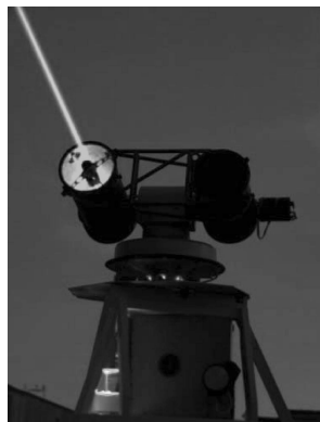
Figure 4: Satellite Laser Ranging System “Sazhen-TM”. Satellite heights 400–23000 km, optical system diameter 25 cm, laser pulse frequency 300 Hz, pulse energy 2.5 mJ, mass 120 kg, normal points precision 1 cm, angular precision 1–2”.
