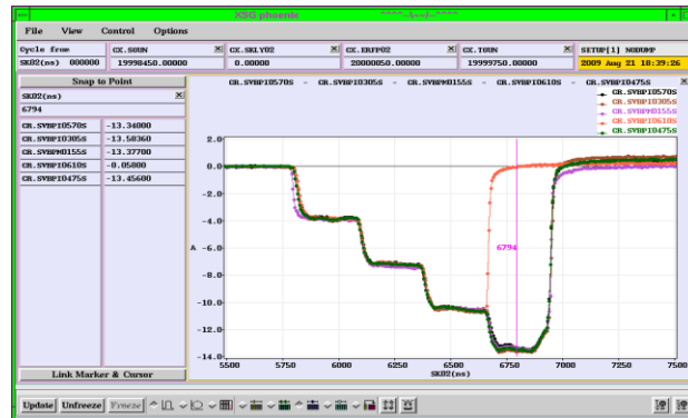
Figure 4. Recombination by a factor of four in the CTF3 combiner Ring. The beam current as a function of time in the first two Beam Position Monitors is shown.
