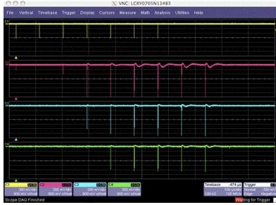
Figure 1: BPTX signal (yellow) with MBTS signals (pink, blue, green) show synchronised behaviour during single beam running.
