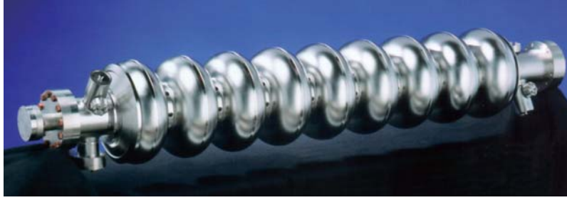
Fig.1: Solid Nb nine-cell cavity as foreseen for ILC
