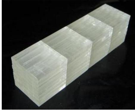
**Figure 3:** Photograph of stacked crystals for a prototype calorimeter composed of 160 GSO(Ce) crystals of  $4 \times 6 \times 30 \text{ mm}^3$ .
