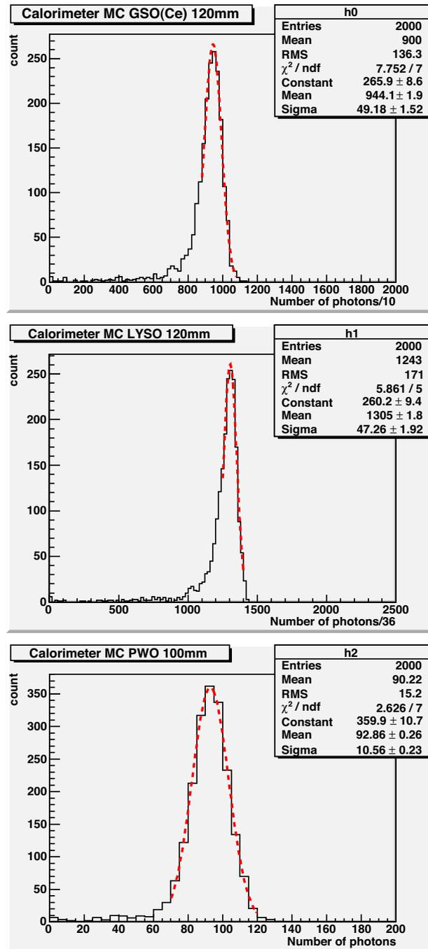
**Figure 9:** Distributions of the number of photons arrived at the photon detectors for GSO(Ce) (top), LYSO (middle), and PWO (bottom). The number of photons emitted by the scintillation process is reduced by some factors.
