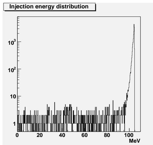
**Figure 8:** The energy distribution of electrons, which are injected to the calorimeter.
