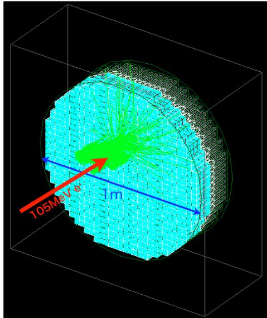
**Figure 6:** A typical event display of the simulation study of the calorimeter. An electron injected to the calorimeter, then optical photons from scintillation processes are ray-traced to the photon detectors.
