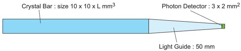
**Figure 7:** A schematic view of a segment of the calorimeter used in the simulation study.
