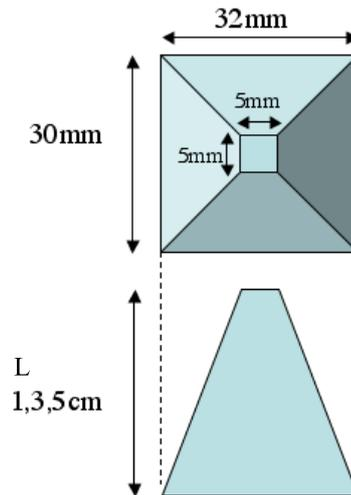
**Figure 4:** Drawing of the light guides connected to the stacked GSO(Ce) calorimeter.
