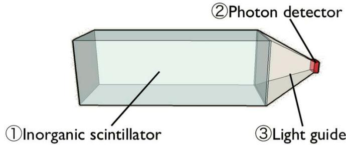
**Figure 2:** Conceptual design of a segment of the calorimeter.
