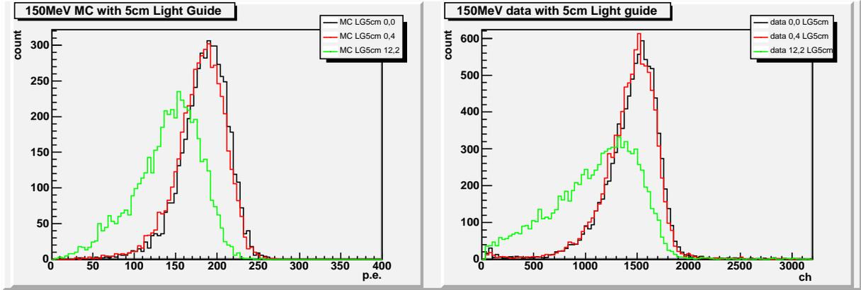
**Figure 5:** Distribution of the number of photons for 150 MeV electrons injected with  $L=5$  cm light guide case: left histograms are by Monte-Carlo simulation and right histograms are from the beam test. Each of three histograms shows injection position of the beam:  $(x[\text{mm}], y[\text{mm}])=(0,0),(0,4),(12,2)$ . The position  $(0,0)$  means the center of the stacked calorimeter.
