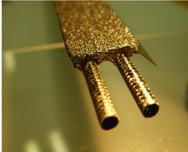
**Figure 5:** Prototype of a full carbon fibre homogeneous stave. Two carbon fibre pipes, which are fully qualified for the IBL usage have been integrated into the carbon foam.
