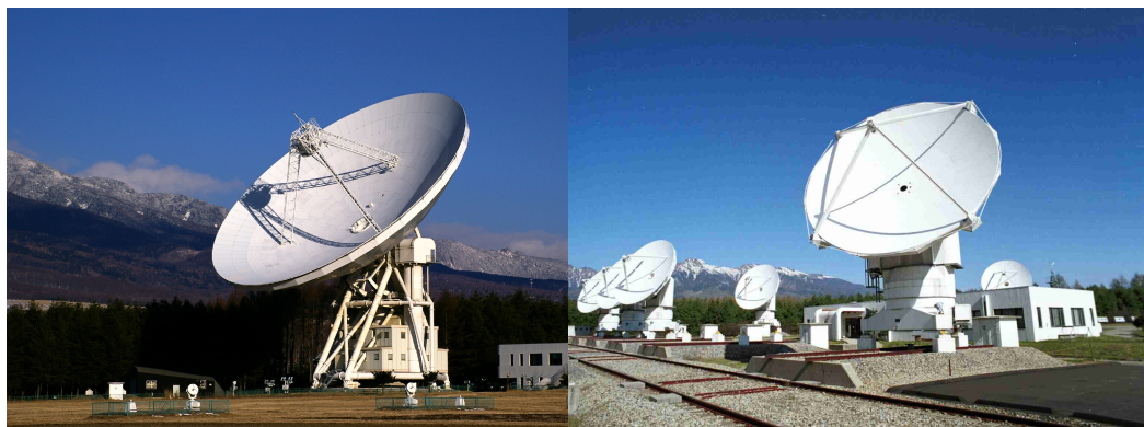
Figure 2. Nobeyama mm-wave telescopes: 45-m telescope (left) and 5-element interferometer (NAOJ).
