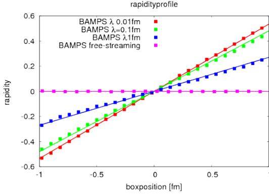
**Figure 3:** rapidity gradient in BAMPS with  $y_{wall} = 0.55$ ,  $Boxlength = 2$  fm and variable  $\lambda_{mfp}$ . Comparison with results from Eq. (4.4).
