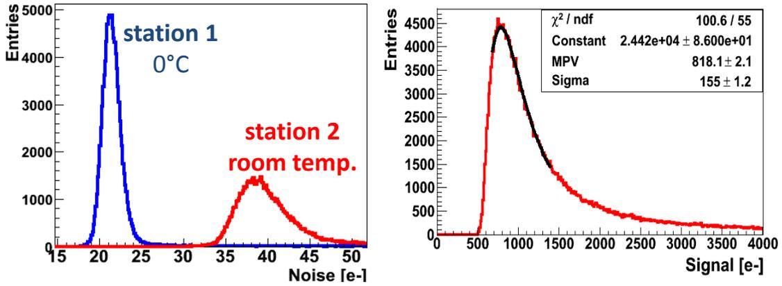
**Figure 2:** Noise averaged (left) of each pixel over 500 frames during the beam test for station 1 cooled down to 0 °C and for station 2 running at room temperature. The signal distribution (right) of the demonstrator for a  $3 \times 3$  cluster including the seed pixel. The signal cut was set to 5 times the average noise (i.e.  $\sim 110 \text{ e}^-$ ).
