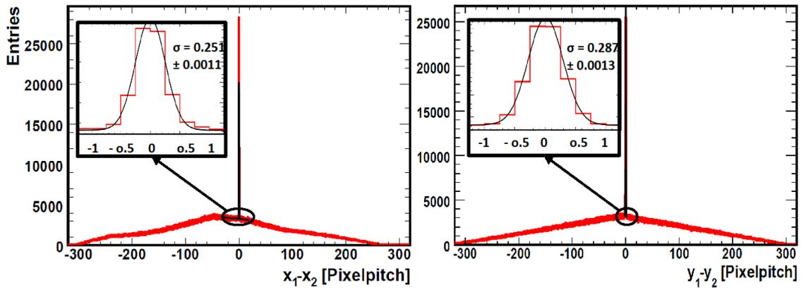
**Figure 3:** Position residual plot of the two demonstrator stations in x- (left) and y- (right) coordinate with a pixel pitch of  $30 \mu\text{m}$ . The zoomed insert shows details of the position correlation, together with a gauss fit.
