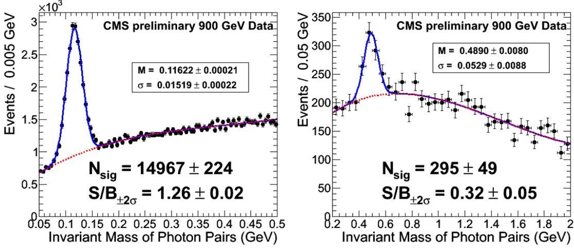
**Figure 2:** Left: Invariant mass spectrum of photon pairs in ECAL barrel with  $E_T(\gamma) > 300$  MeV and  $E_T(\pi^0) > 900$  MeV, with uncorrected energies. Right: Invariant mass spectrum of photon pairs in ECAL barrel with  $E_T(\gamma) > 400$  MeV and  $E_T(\eta) > 2$  GeV, obtained with  $\pi^0$  veto and uncorrected energies.
