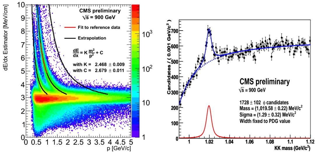
**Figure 4:** Left:  $dE/dx$  versus  $p$  in data collected at 0.9 TeV, during the December 2009 run. The red line gives a fit with proton mass assumption, in a restricted  $p$  range, while black lines show extrapolations. Right: Fit to the mass distribution of kaon candidate pairs in data. The natural width is fixed to the value of  $\Gamma_{\phi(1020)} = 4.26 \text{ MeV}/c^2$ .
