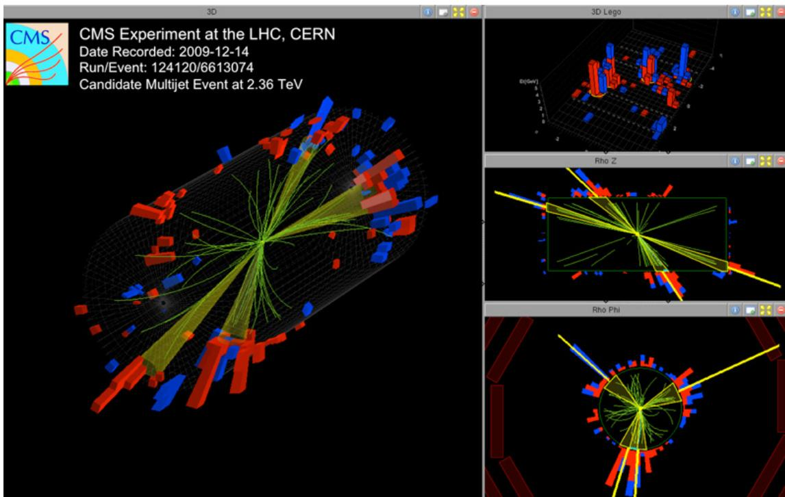
**Figure 1:** A reconstructed 2.36 TeV proton-proton event with tracks and calorimeter towers.
