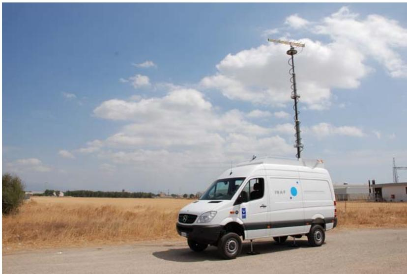
*Figure 1 – SRT’s mobile station with a log-periodic antenna placed on the pole.*
