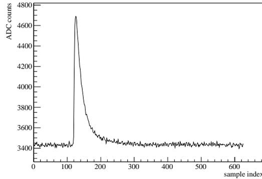
**Figure 2:** Signal produced by an 88 keV  $\gamma$  particle fully absorbed in one detector. The signal is sampled at 125 Hz and the length of the window corresponds to 5.008 s.
