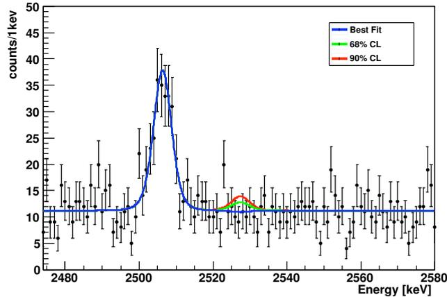
**Figure 1:** CUORICINO energy spectrum in the region of interest. The line at 2505 keV is due to  $^{60}\text{Co}$  contamination of the materials surrounding the bolometers. No peak is found at the expected  $0\nu\text{DBD}$  energy of 2527 keV.
