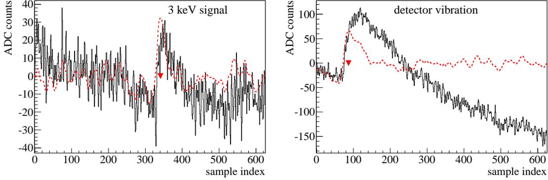
**Figure 3:** Windows of data samples containing pulses. The raw data (solid black line) have been shifted such that the first sample has zero ADC counts; the filtered data (dashed red line) are not modified. Red triangles identify the pulses detected by the trigger algorithm. The filter removes the baseline drifts and suppresses pulses with different shapes than the expected signal.
