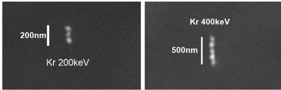
Fig.2 Scanning electron microscope (SEM) image of low velocity Kr ion (200 and 400keV) tracks demonstrated the nuclear recoil tracks. White spheres are silver grains generated by development treatment. This line reflects the track of an ion (or a recoil nucleus).
