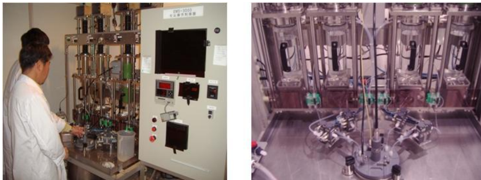
Fig.6. The installed machine to produce the nuclear emulsion in laboratory.
