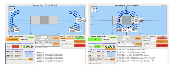
**Figure 2:** Screenshots of the PVSS closing manager, showing the VELO in the retracted position (left) and then after closing (right). This panel updates in real-time during the closing procedure.
