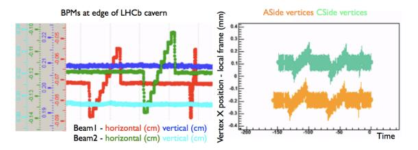
**Figure 4:** During a Van der Meer scan, the movement of the two beams in the horizontal plane (seen in the BPMs, left) manifests itself as a change in the x position of the reconstructed vertices (right). The offset between A and C side vertices is due to measurements being made in the local frame of each half.
