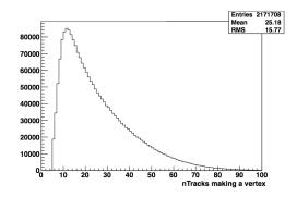
**Figure 5:** Number of tracks making a vertex in beam-beam events. An average vertex is made of 25 tracks. The highest number of tracks making vertices is around 80, which makes it difficult to calculate the resolution above 40 tracks as the total number of tracks must be split in two.
