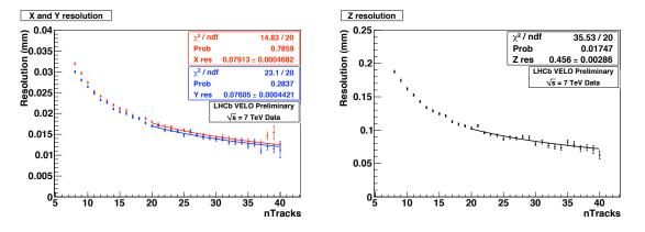
**Figure 6:** Resolutions as a function of track multiplicity in data. The data points are fitted between 20 and 40 tracks with the function  $\sigma_{\text{res}} = \sigma_0 / \sqrt{N}$ , where  $\sigma_0$  is the fitted constant and *N* is the number of tracks.
