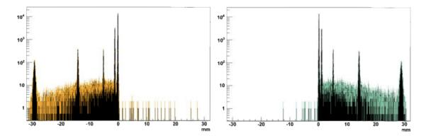
**Figure 3:** The closing as seen through the eyes of the VELO, with vertex positions reported in the local frame of each half. The positions where the VELO paused ( $\pm 29$ ,  $\pm 14$ ,  $\pm 5$ ,  $\pm 1$ , 0 mm) are clearly visible.
