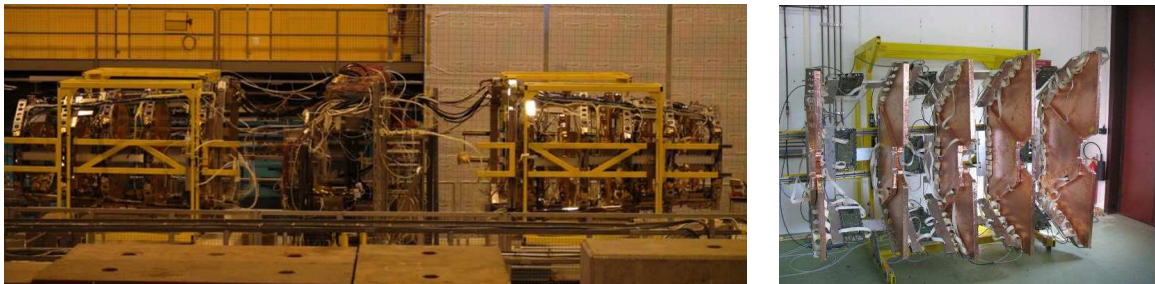
Figure 2: The full T1 detector during the beam tests in the SPS experimental area (left) and a quarter (right).
