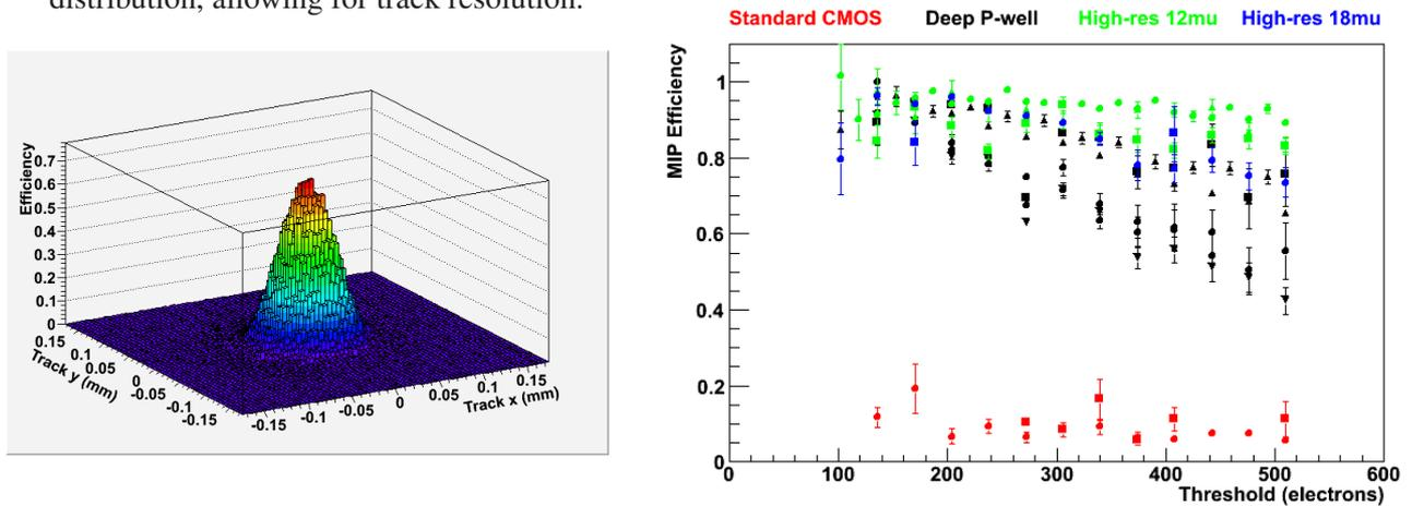
**Figure 2:** Left: Typical distribution for the probability of a hit as a function of position relative to the track projection. Right: MIP efficiency as a function of threshold, for all four sensor variants.
