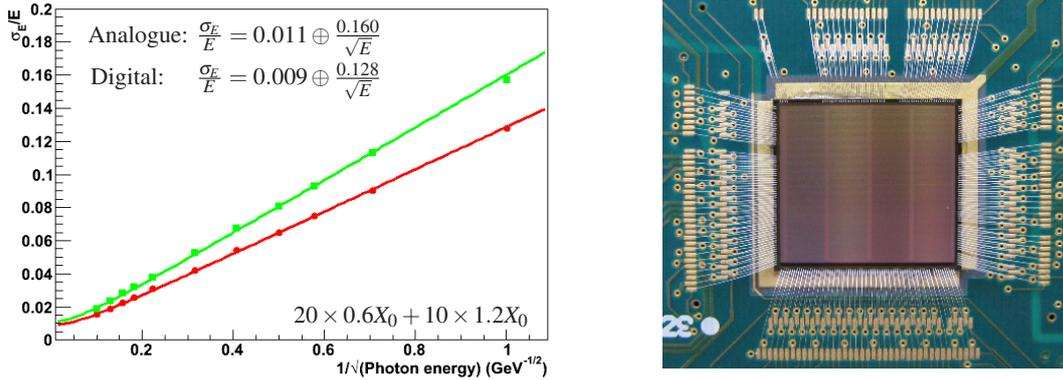
**Figure 1:** Left: Comparison of  $\sigma_E/E$  as a function of  $1/\sqrt{E}$  for simulated analogue (green) and digital (red) electromagnetic calorimeters with a typical ILC geometry. Right: Photograph of a TPAC V1.2 sensor.
