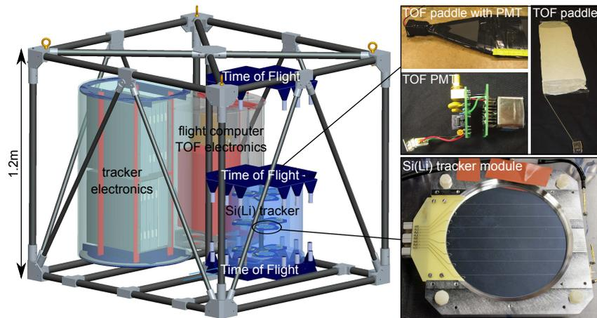
**Figure 3:** Prototype GAPS experiment with detailed views of the time of flight system and the Si(Li) tracker modules.
