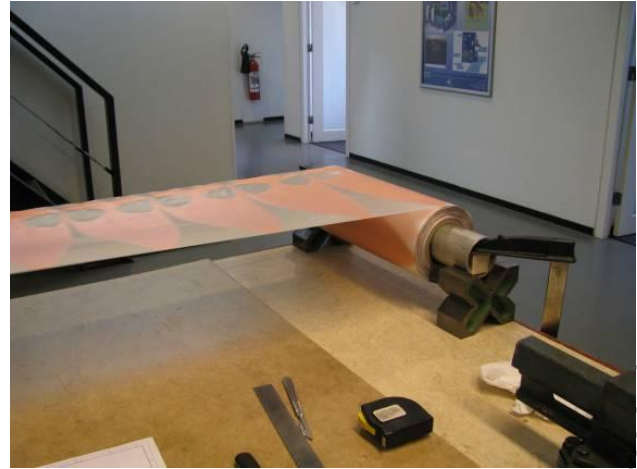
Fig. 5: Foil based vivaldi on roll
