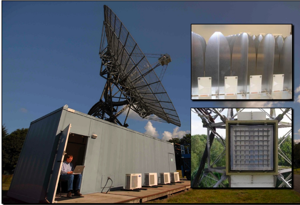
Fig. 1: The WSRT telescope RT5 equipped with the APERTIF prototype. Shown in the inserts is the Vivaldi array in the lab (top right) and in the focal plane of the telescope (bottom right).
