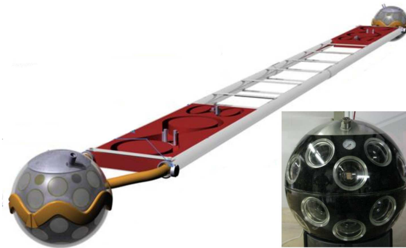
Figure 1: Artistic illustration of a DOMBAR Unit. The distance between the DOMs is 6 meters. A prototype of the Digital Optical Module is also shown.
