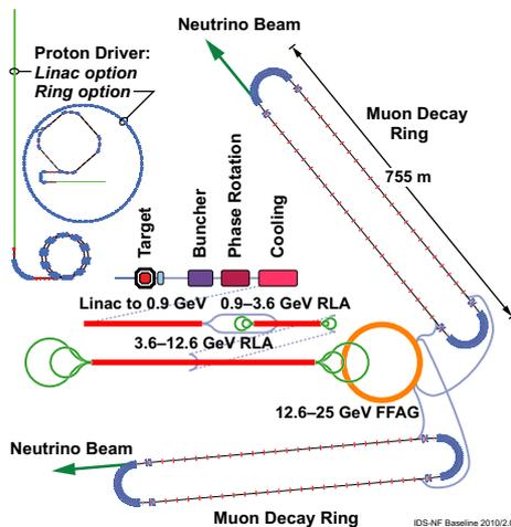
**Figure 1:** Schematic drawing of the IDS-NF accelerator complex.
