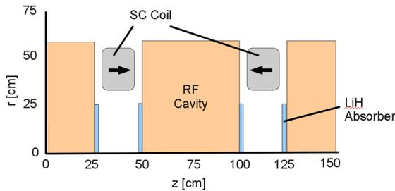
**Figure 3:** Baseline design of muon cooling lattice.
