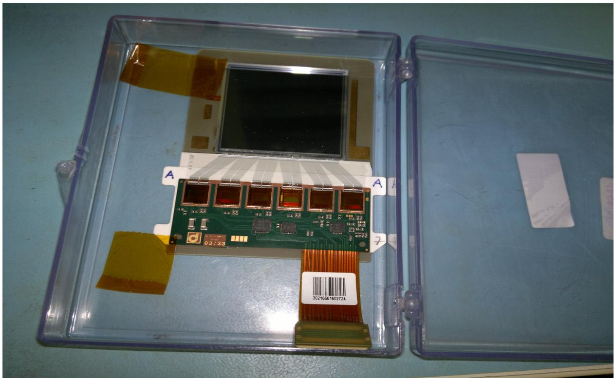
Mechanical failure has been seen in a sensor module with ceramic support, as shown:
