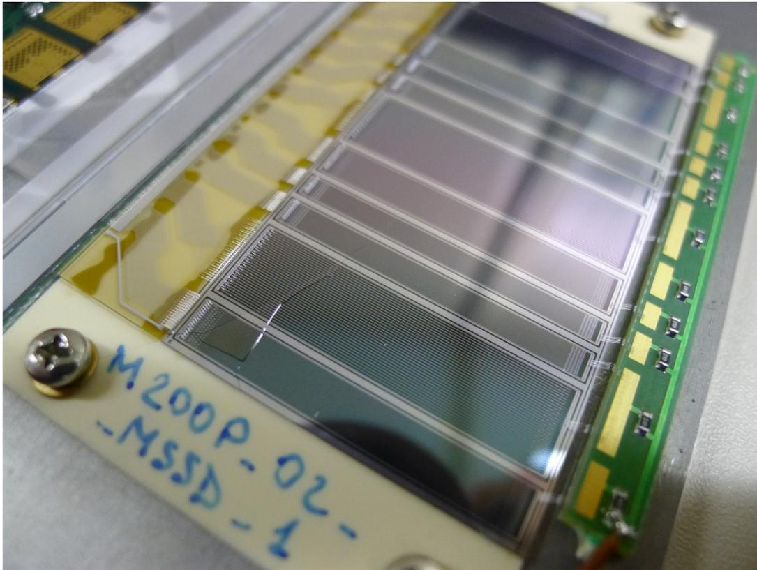
This cracked sensor module is not a CID and the crack is (most likely) occurred when the irradiated module has been taken out  $-20^{\circ}\text{C}$  freezer.
