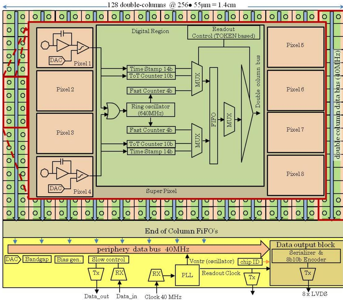
Figure 1. Top level block diagram of Timepix3 chip
