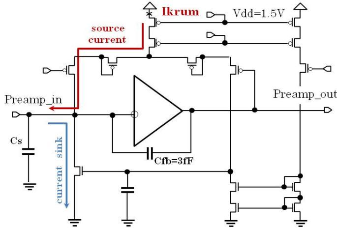
Figure 4. Schematic of the preamplifier circuit
