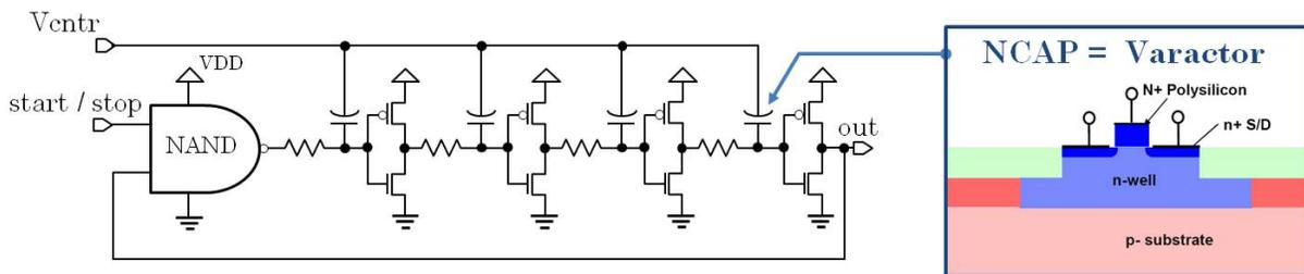
Figure 3. The start-stop ring oscillator implemented in the TDC
