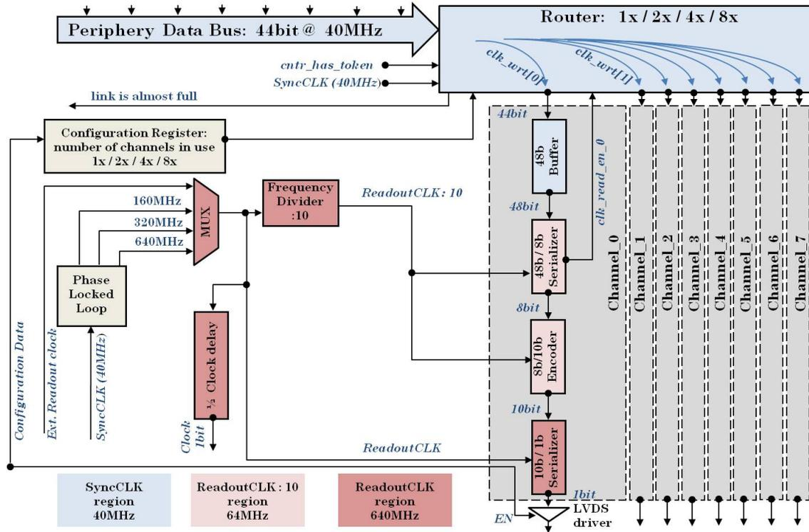
Figure 5. Block diagram of the Output block in the Timepix3
