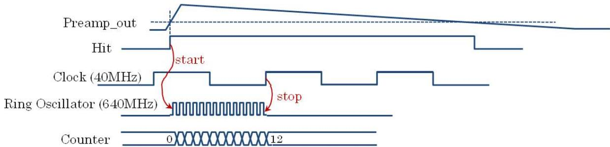
Figure 2. Signals in the TDC based on concept of the start-stop ring oscillator
