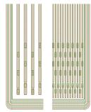
Figure 6: Multi geometry strip sensor for optimizing layout parameters.
