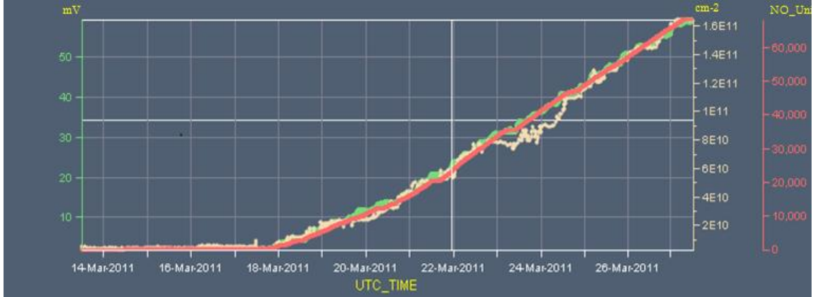
Fig. 5: RadFET signal (mV), \Phi_{eq} ( n_{eq}/cm^2 ) and SEU counts are respectively illustrated in green, beige, red getting from Timber. The SEU counters are used to evaluate the HEH and thermal neutron fluence as described in [15].
