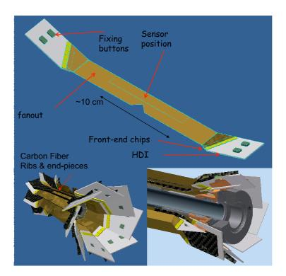
**Figure 2:** Drawings of the octagonal Layer0 made of striplets modules. In the inset, the striplet modules positioned on the cold flanges with the Be beam-pipe.
