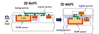
**Figure 4:** Schematic concept of 2D MAPS, with DNW sensor on a single CMOS tier, and 3D MAPS realized with two CMOS tiers interconnected.
