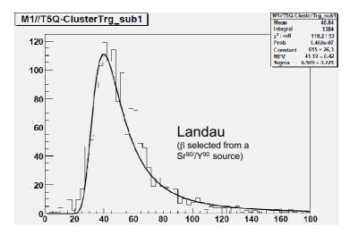
**Figure 5:** Cluster signal of the 3x3 MAPS matrix with a  $^{90}$ Sr  $\beta$  source.
