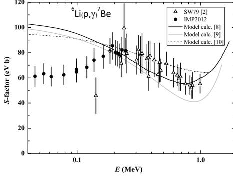
**Figure 3:** Astrophysical  $S$ -factor data of  ${}^6\text{Li}(p, \gamma){}^7\text{Be}$ . The triangle data points are from previous work and the solid points from present work. The solid line represents previous theoretical calculation results [8–10].
