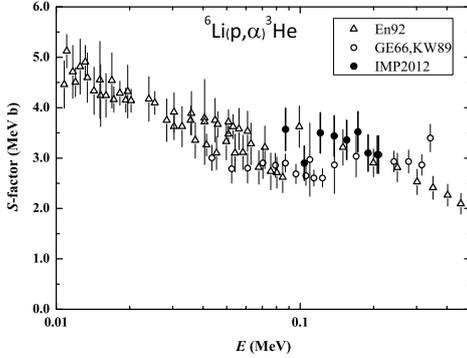
**Figure 4:** Astrophysical  $S$ -factor data of  ${}^6\text{Li}(p, \alpha){}^3\text{He}$ . The solid data points are from present work. The previous data are also shown for comparison, where the triangle data points are from [12] and the hollow circles from [15, 16].
