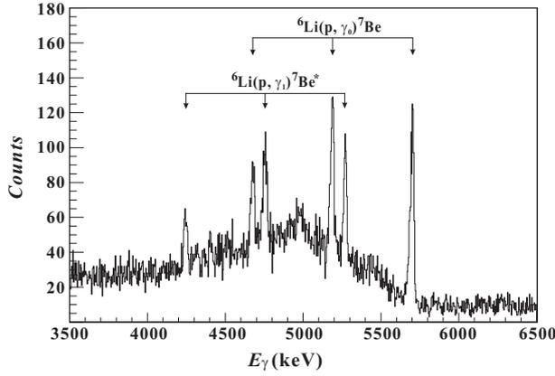
**Figure 1:** Sample  $\gamma$ -ray spectrum from the  $p+{}^6\text{Li}$  radiative capture reaction obtained at energy of  $E=94$  keV.
