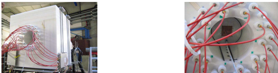
Figure 2: (Left) Picture of the BELEN detector as it was set-up at the S4 experimental hall. (Right) Closer view of the central hole where the SIMBA detector was placed.
