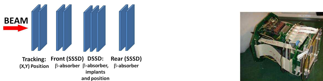
Figure 1: Schematic view (left) and picture (right) of the SIMBA detector.
