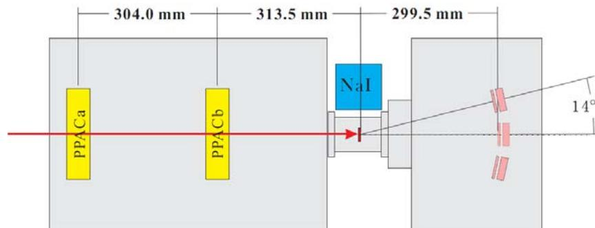
**FIGURE 1.** Schematic view of the detector setup at F3 focal plane of CRIB.
