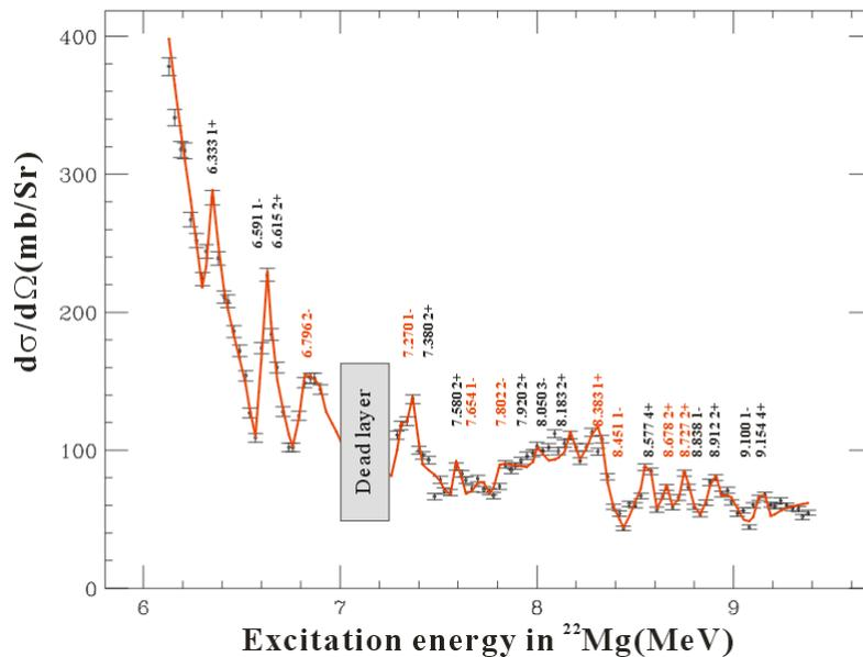
**FIGURE 3.** Elastic-scattering proton spectrum with a typical R-matrix fitting (Preliminary).
