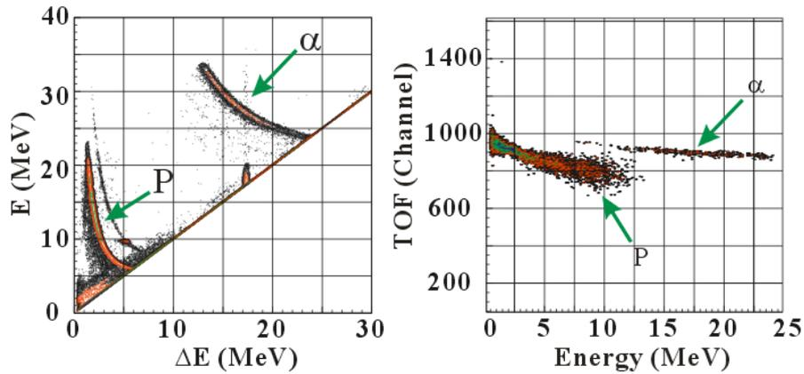
**FIGURE 2.** Particle identification plots for the  $\Delta E$ -E and E-TOF methods. The start TOF signal is given by PPACa, and the stop signal is given by  $\Delta E$ .
