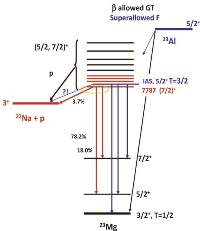
**Figure 3.** Partial decay scheme of  $^{23}\text{Al}$ . Only the transitions to the first 3 levels of daughter nucleus  $^{23}\text{Mg}$  are shown in the lower part to justify the spin and parity assignment of its ground state. The decay of the doublet around  $E^*=7.8$  MeV (the IAS and the  $E=7787$  keV state), including a 3.7% proton branch is also shown. It is very rare that the decay of a state by both gamma-ray and proton emission is observed.
