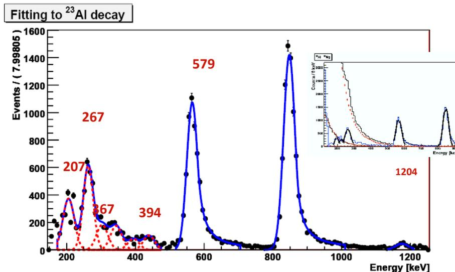
**Figure 2.** Proton spectrum following the  $\beta$ -decay of  $^{23}\text{Al}$  measured with a 65  $\mu\text{m}$  DSSSD (from Ref. [4]). Note in the insert the high background which is attributed to the betas, as are the tails of the proton peaks.
