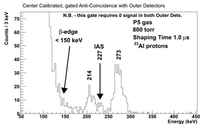
**Figure 4.** Zoom of calibrated spectrum for the low energy p spectrum of  $^{23}\text{Al}$  measured with AstroBox. The energies marked are c.m. energies (preliminary calibration and analysis).
