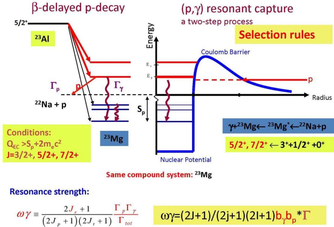
**FIGURE 1.** (Color online) Schematic presentation of the use of  $\beta$ -delayed proton decay to study resonant H-burning in nuclear astrophysics.
