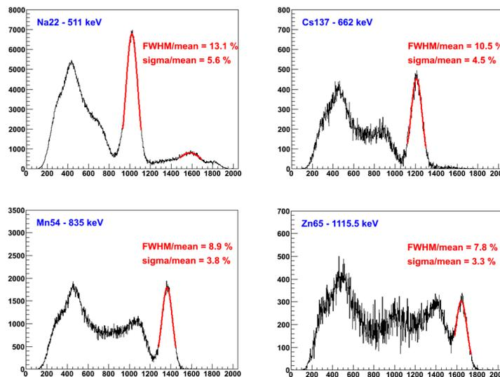
**Figure 4:** Amplitude spectra of different  $\gamma$  sources from (LYSO+SiPM), measured at an overvoltage of 5.4 V.
