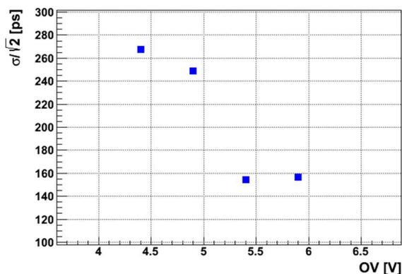
Figure 6: CRT resolution as a function of the overvoltage.
