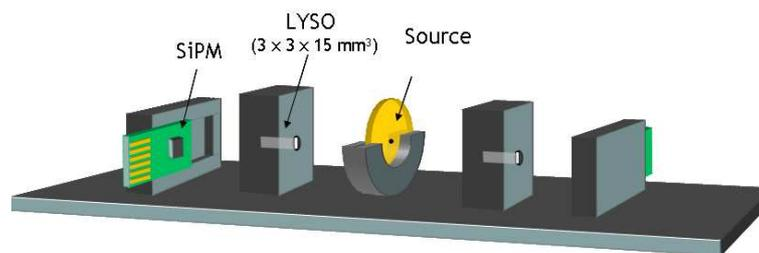
Figure 1: Layout of the experimental set-up.
