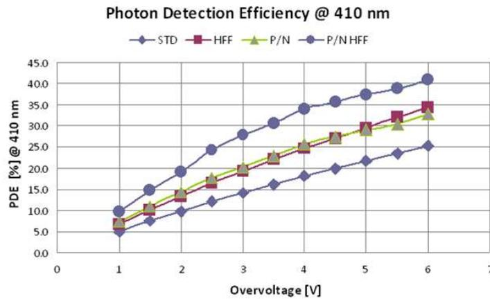
**Figure 3:** Comparative measurements of Photon Detection Efficiency for different STMicroelectronics devices. STD= Standard Process, HFF=High Fill factor process, P/N= "p on n" Process, P/N HFF="p on n" High-Fill Process, suitable for TOF PET. Accuracy for such measurements is around 10%.
