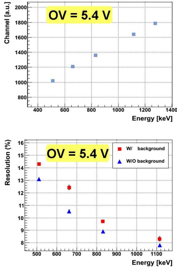
**Figure 5:** Photopeak positions (top) and resolution - with and without the background - for the various gamma energies, at an overvoltage of 5.4 V
