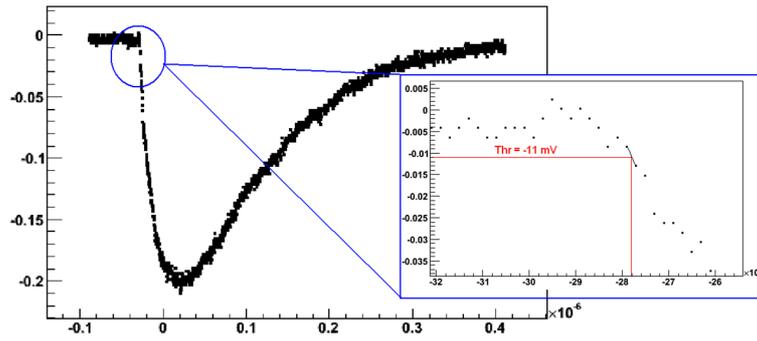
**Figure 2:** A typical signal from one of the devices under test. The insert shows the beginning of the signal, which is critical for the time resolution.
