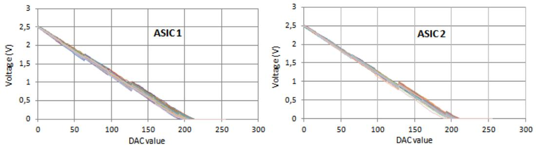
Figure 5: 8-bit DAC linearity
