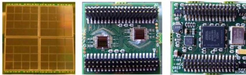
Figure 3: SiPM board (a), ASIC board (b) and FPGA board (c)
