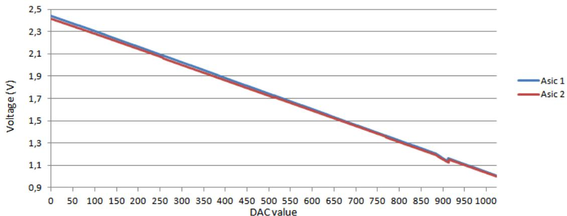
Figure 6: 10-bit DAC linearity
