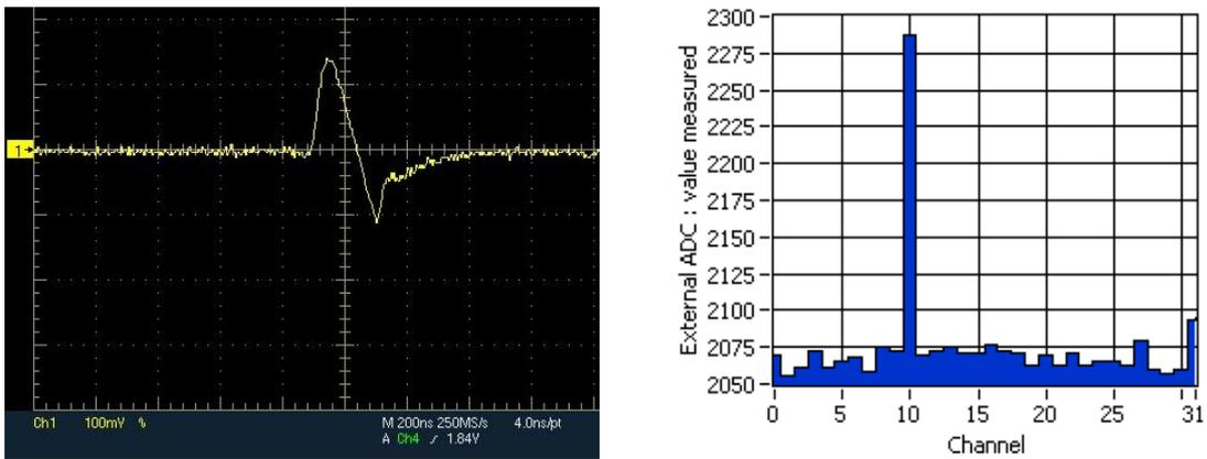
Figure 7: Scope screenshot of slow shaper HG output for a fixed injected charge of 1.6 pC (left) and the corresponding live ADC acquisition (right)
