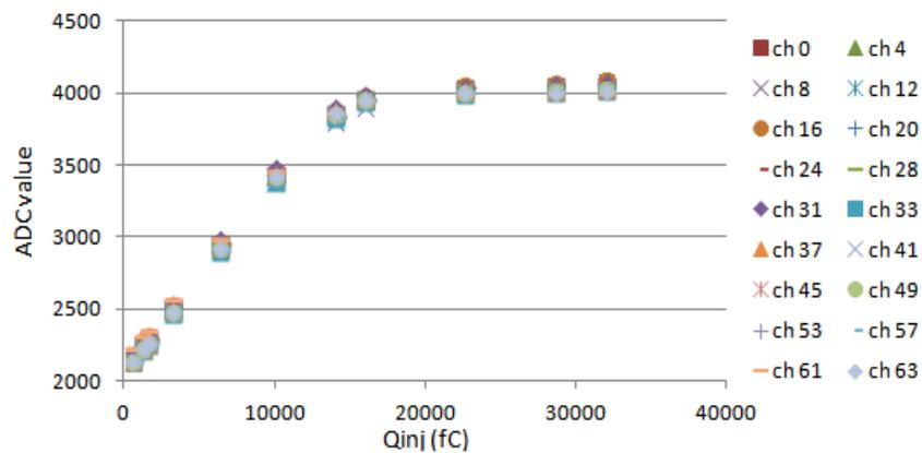
Figure 9: high gain versus injected charge
