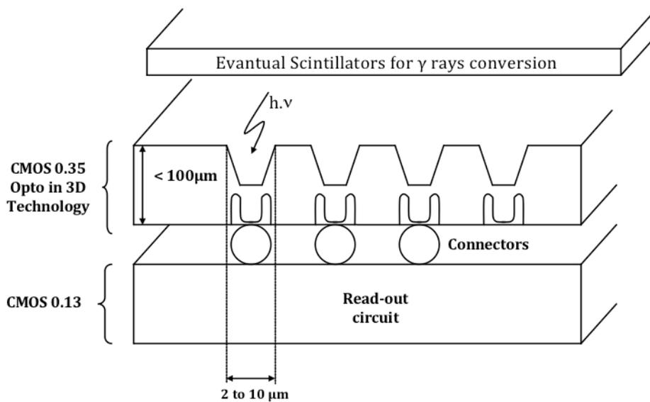
**Figure 4:** Proposed structure in 3D technology. Top layer includes photodiode structures; bottom layer includes read-out circuits for signal treatments.
