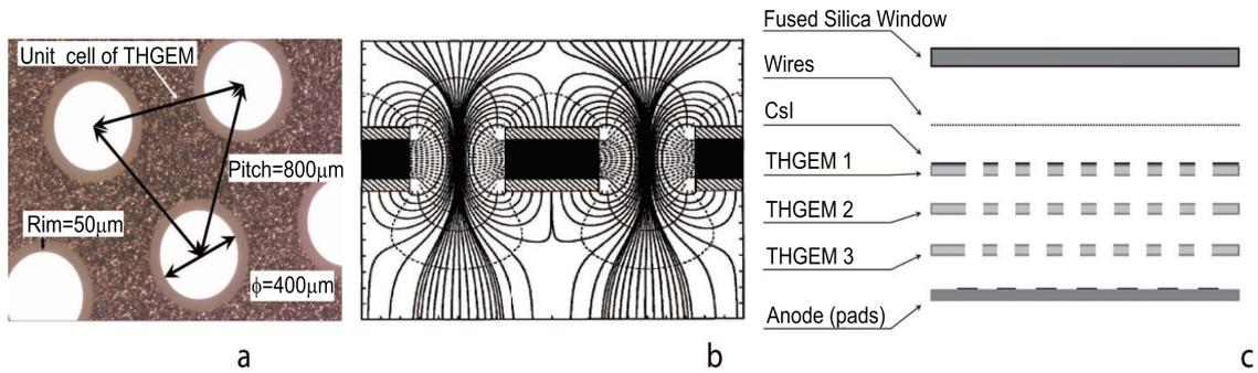
**Figure 1:** a: Image of a THGEM detector; the main geometrical parameters namely the holes diameter, the pitch and the rim are indicated. b: Field lines obtained by a calculation exercise. c: Sketch of a triple THGEM photon detector arrangement (not to scale).
