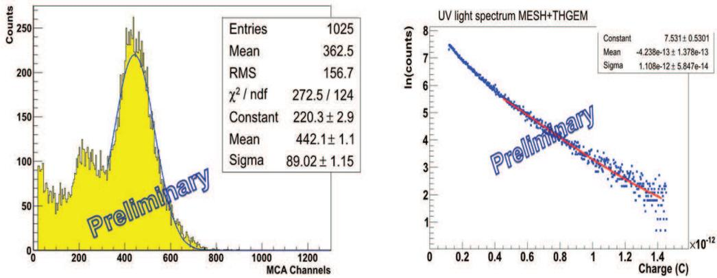
**Figure 3:** Amplitude spectra obtained with the hybrid detector prototype. Left: using the <sup>55</sup>Fe source; estimated gain:  $2.5 \cdot 10^5$ . Right: illuminating in single photon detection mode; estimated gain:  $\approx 1.2 \cdot 10^6$
