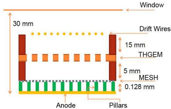
**Figure 2:** Scheme of a hybrid detector (not to scale). The geometrical parameters refer to the detector used to obtain the results presented in sec. 3
