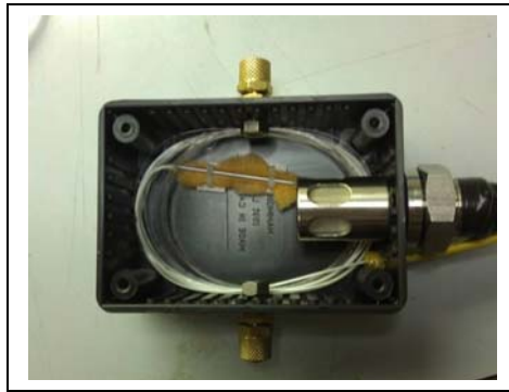
Fig.2. FBG sensor arranged in the box with T and RH reference monitoring sensors.
