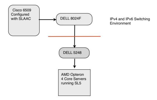
This test deployment was designed to emulate the hardware deployed within the GU Scotgrid production cluster in 2011. The module used to connect to the Campus network was a 1 Gigabit Long Reach SFP connected via multimode OM3 fibre into the 8024F.
