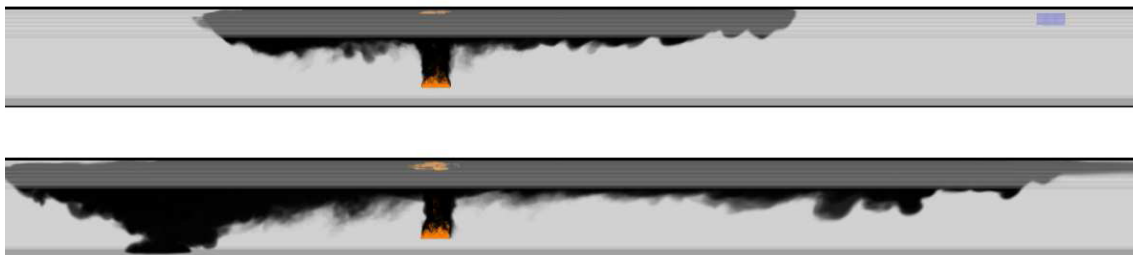
Fig. 2 Smoke development at the 50 th and 57 th second of fire
