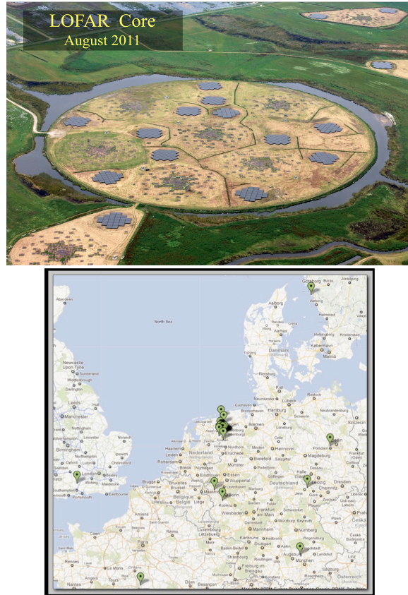
Figure 3. Top: The LOFAR Superterp is the innermost area, densely packed with the hardware of 6 stations. It is surrounded by several of the innermost core stations, visible as separate patches. Bottom: the locations of the current 8 international LOFAR stations in relation to the concentration of stations in the Netherlands.
