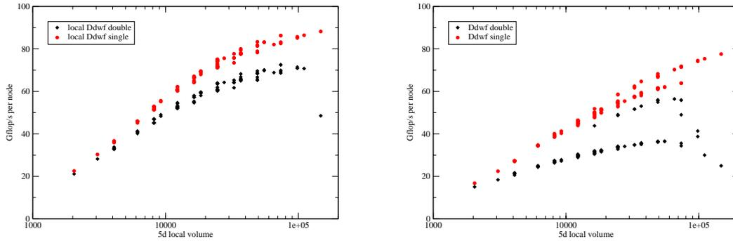
**Figure 10:** Left: single node application of  $D_W$  to  $L_S$  fermion fields. This is a key component of chiral fermion simulations, and contains around 90% of the floating point operations. L2 spillage occurs for 5d volumes greater than around  $10^5$  sites. Right: multi-node application of  $D_W$  to  $L_S$  fermion fields. In double precision the communication impact of different aspect ratios for the local volume is visible.
