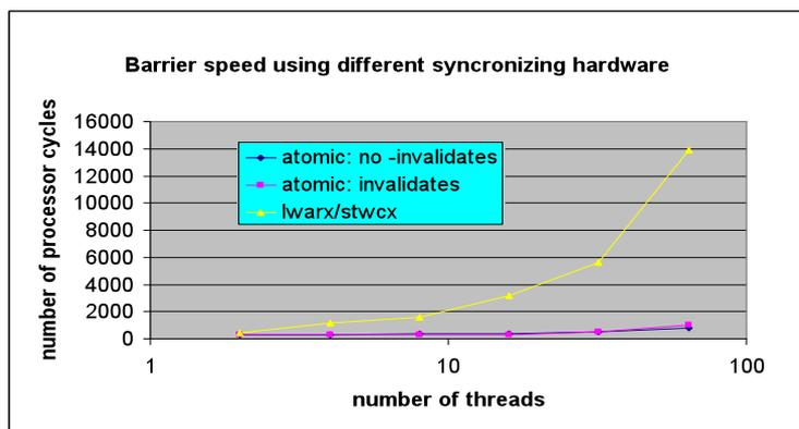
**Figure 6:** With up to 64 threads on each compute node, fine grained threading performance is important. BlueGene/Q provides hardware assistance for interthread synchronisation with hardware atomic operations on any memory address. This avoids, for example, costly load-locked/store-conditional synchronisation to access a shared barrier variable, and accelerates synchronisation substantially.
