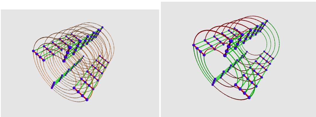
**Figure 9:** Here some solutions used by the author to fill a  $4 \times 4 \times 6$  (radial-mesh, azimuthal-torus, axial-mesh). Left plot: the unmodified 3d mesh-torus-mesh displaying all physical links. Right plot: the links used to embed a  $8 \times 12$  application torus (red,green) in this 3 dimensional space. Code implementing these mappings has been provided to the maintainers of QMP.
