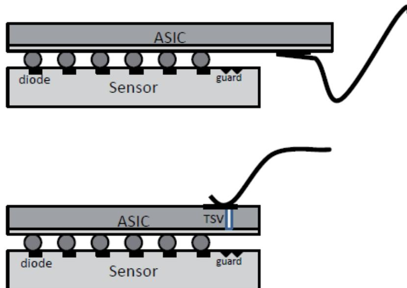
**Figure 3:** Top: State of the art layout of a hybrid pixel detector (Readout ASIC bump bonded onto a pixel sensor). In order to access the I/O pads of the chip it has to cantilever beyond the sensor causing dead space. Bottom: Using TSV the I/O can be routed to the backside of the chip making the cantilever obsolete.
