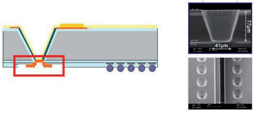
**Figure 5:** Left: Routing of the I/O to the back side of the chip using tapered, copper lined vias. The vias are etched through the bulk from the backside and connected by a copper plug. Right: Pictures of tapered vias processed by Fraunhofer IZM (Courtesy University of Bonn/IZM, Berlin)
