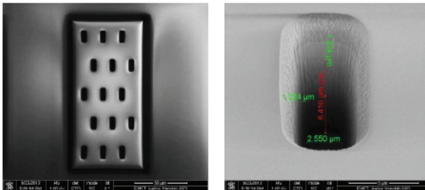
**Figure 4:** TSVs etched by EMFT into the ATLAS FEI3 chip. In order to have a redundant insulation of the vias from the bulk a protecting trench is etched around the vias. The via dimension is  $2.5\mu\text{m}$  times  $5\mu\text{m}$ .
