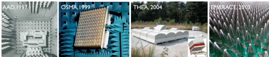
Figure 3: Four generations of ASTRON's Aperture Array tile development programme - from the early 1990s through to the present day. Images courtesy, A. van Ardenne, J.G. bij de Vaate (ASTRON).
