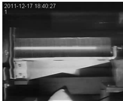
Figure 9: Finite range (30 cm ca) of extracted carbon beam through a plastic scintillator at 455 MeV/u.
