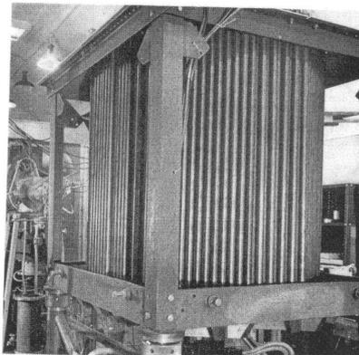
Figure 1: General view of the ADS assembly [5] showing the 99 cm diameter and 107 cm height pile. The effective uranium density is  $\rho = 16.3 \text{ g/cm}^3$ .
