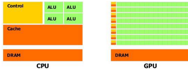
Figure 4: Structural difference CPU – GPU
