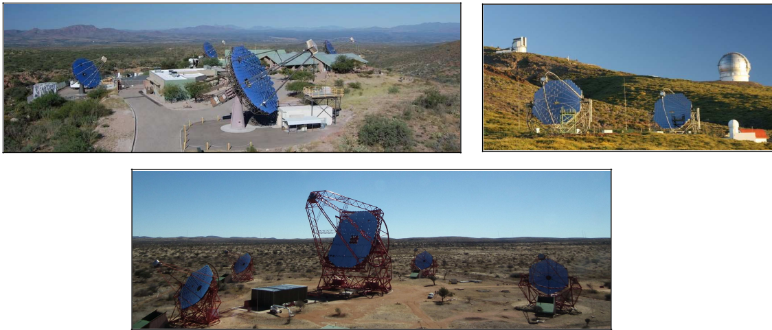
Figure 1. The three main current ground-based Imaging Atmospheric Cherenkov Telescopes, VERITAS (Very Energetic Radiation Imaging Telescope Array System, Arizona), MAGIC (Major Atmospheric Gamma Imaging Cherenkov Telescope, Canary island of La Palma) and HESS (High Energy Stereoscopic System, Namibia), with the new HESS II telescope (28 m).
