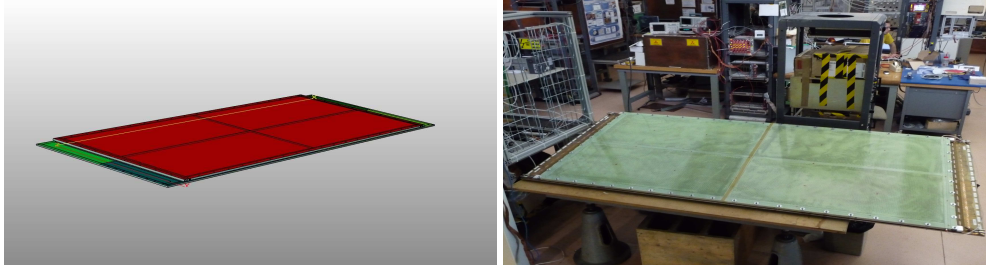
Figure 3: The 3D rendering and a picture of the large Micromegas chamber after the assembling.
